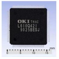
The ML610Q400 series is capable of operating at only 1.1 V,
